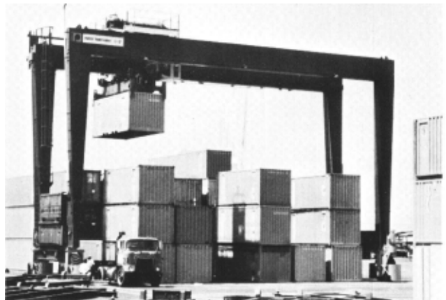
PACECO MACH Transtainer systems for handling containers in the yard.
