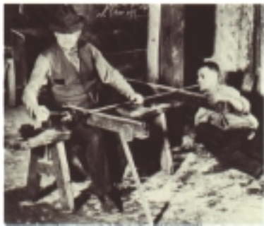
AT THE TURN OF THE CENTURY, A TEAM OF TWO MEN COULD PRODUCE THREE GLASS BULBS PER MINUTE.
