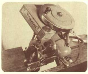
'R' — This 1917 model was the first Evinrude with 360degree reverse steering and tilting too. Full forwardneutral-reverse shifting was to come later.
