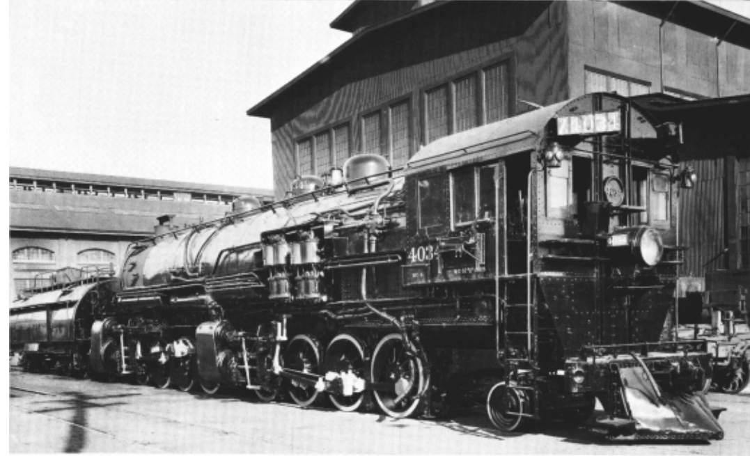
Southern Pacific's first cab-in-front (top) shows the original compound articulated engine after cylinder conversion to single expansion H.P. #4034 (above) was one of the first Mallet consolidated (double expansion) cab-in-front engines. #4272 (below) shows the latest configuration.
