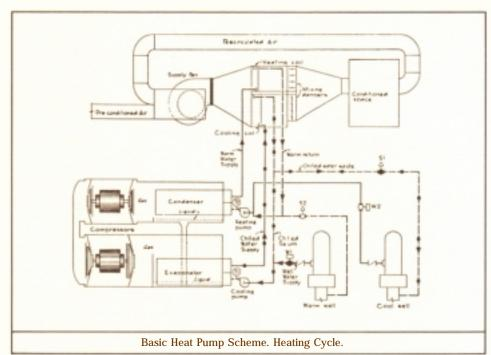
Outside air was not used for the internal or minimum cooling, inasmuch as to do so would have required equipment arrangement on each floor, encroaching on rentable floor space and would have necessitated additional complexity in automatic control.
