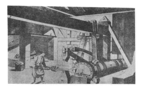
Molten iron flowed from furnace into pig beds (top). Iron being worked at a forge using a trip hammer.
