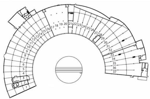
Present day CAD rendering of the Roundhouse. The stalls are numbered as they originally existed in 1924. During the Roundhouse renovation in 1996, stalls 3 and 4 were converted to an orientation gallery. Stalls 17-20 were enclosed for use as exhibit areas, while stalls 21-28 were converted to open space used for renovation of rail equipment.
