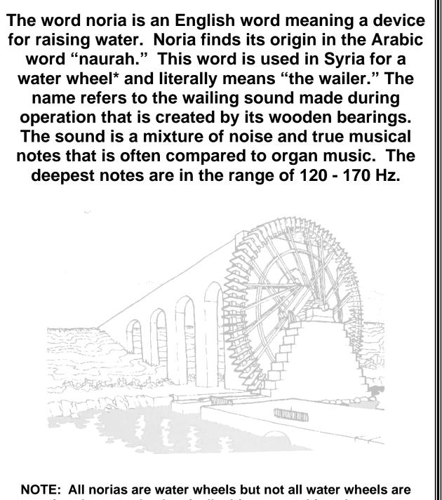
NOTE: All norias are water wheels but not all water wheels are norias. A water wheel typically drives something else e.g. a grindstone, machinery etc. A noria raises water from a stream or river and discharges it at a higher elevation.
