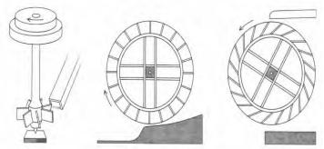
Vertical and horizontal shaft water wheels (Drawing from Scientific American)
