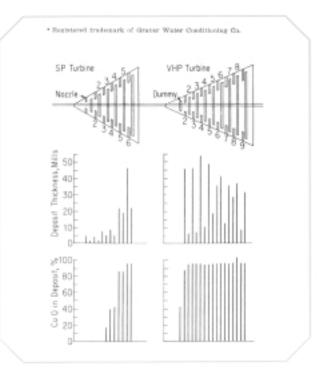
Figure 1.4: Metallic deposits in final stages of SP and all of VHP elements showing high copper content
