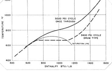
Figure 4: Temperature-enthalpy diagram 5000 psig cycle vs. 2400 psig cycle
