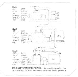
Figure 9: Eddystone feedwater pump arrangement
