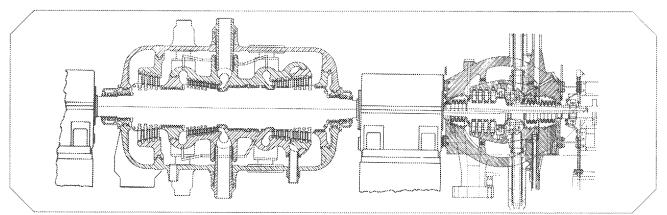
Figure 2: Cross-section of 3600 rpm turbines
