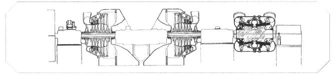
Figure 3: Cross-section of 1800 rpm turbines
