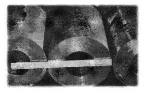
Figure 10: Pipe sections showing massive thickness. Ruler is 18 inches long.
