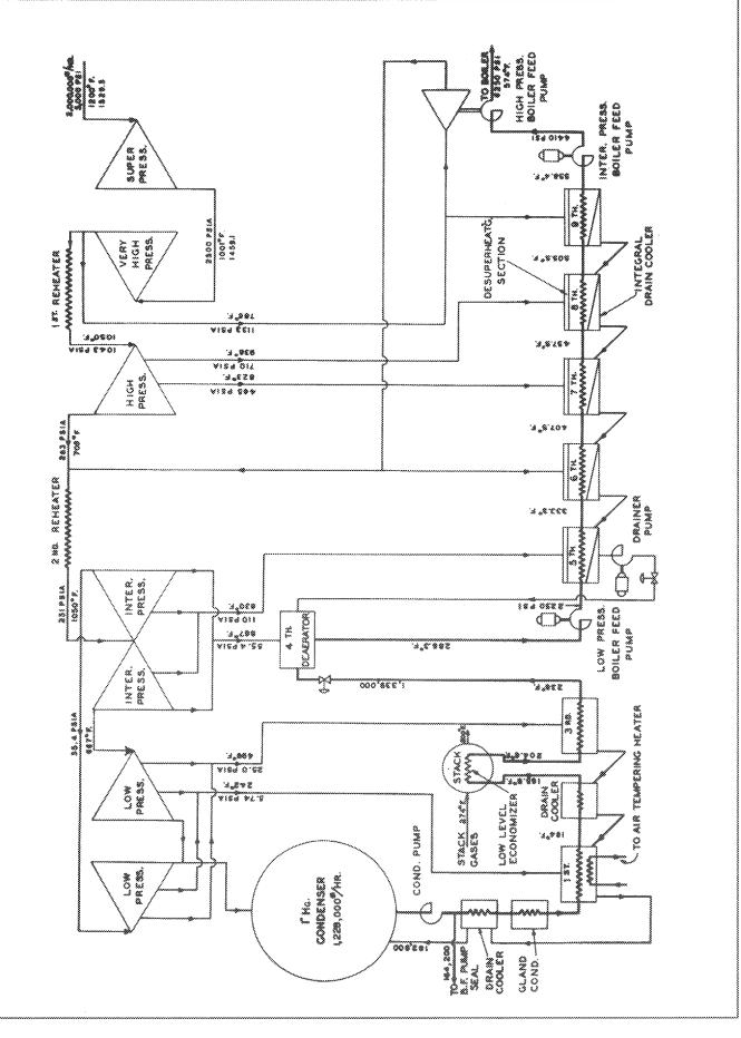
Figure 8: Single - line arrangement of feedwater heaters and pumps
