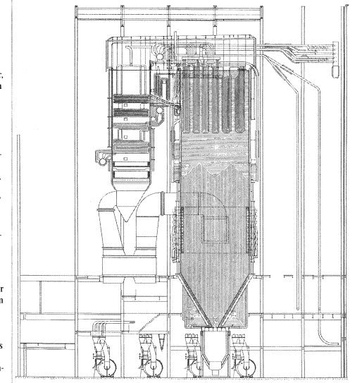
Figure 6: Supercritical pressure steam generator- side elevation
