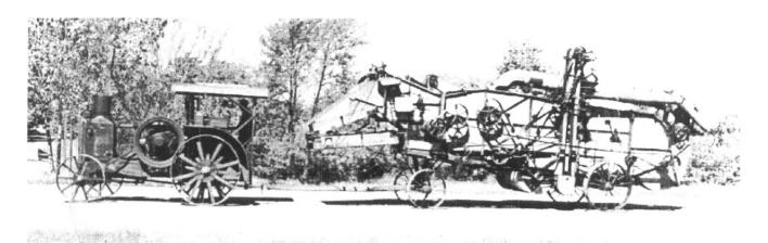
Rumely OilPull Tractor towing steel separator
