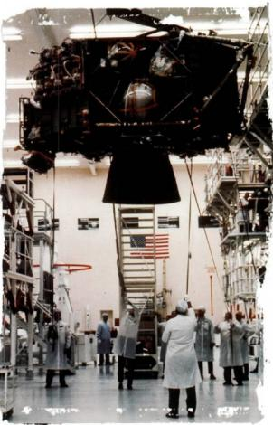
design amounted to something between the two. Because the Lunar Module would be required to perform solely in the space vacuum, engineers could ignore aerodynamic requirements associated with Earth's atmosphere. The result was an aesthetically unappealing, yet functional, spacecraft.
