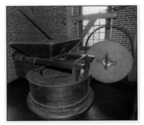
bedstone, which remains stationary during grinding, is fixed in the floor and rests on a special set of beams called stone bearers. An iron drive shaft that holds and turns the upper, or runner, stone comes up through a hole in the center of the bedstone. The runner stone may be raised or lowered as needed to regulate the fineness of the grind.
