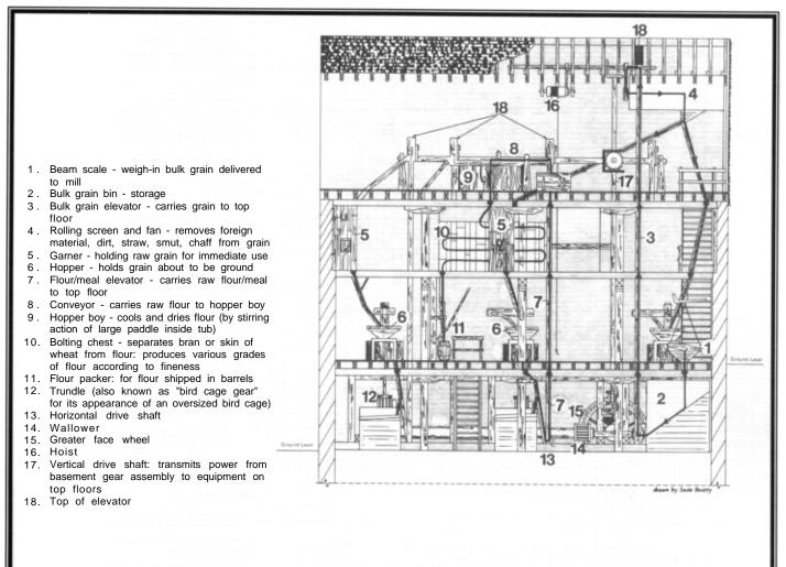
DIAGRAM OF THE MAJOR MECHANISMS OF COLVIN RUN MILL
