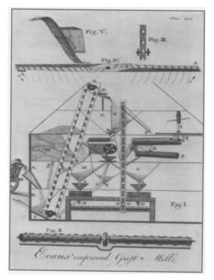
Automation required many mechanical motions and some entirely novel devices invented by Evans, including a mechanical hopper boy, a raking device used to cool flour. Colvin Run Mill exhibits the sole operating hopper boy known in the United States. In combination, Evans' milling innovations boosted output while curtailing labor costs. In the long run, they provided direct precedents for the mass production technologies that came to epitomize American manufacturing.
