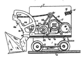
1. In a loading machine, the combination with a support, a horizontally oscillatable superstructure, a vertically swinging shovel mounted on the superstructure, and means for swinging the shovel, of a central cam member mounted on the support, a rotary drum mounted transversely of the superstructure having a cam-edge, and power transmitting means between the shovel swinging means and said rotary drum.
