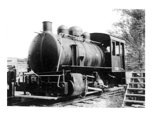
Locomotive #7240 was built by Porter Locomotive Company in 1938. It is one of the newest steam locomotives in existence and is in good condition. The locomotive is a rare "fireless" locomotive with no firebox. It is recharged for operation from a stationary steam plant. This type of locomotive was specifically developed for use in areas where a conventional locomotive would be a hazard with an open fire, such as a refinery or petrochemical plant.
