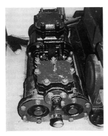
Engine #26 Duplex Cylinder Feedwater Pump
