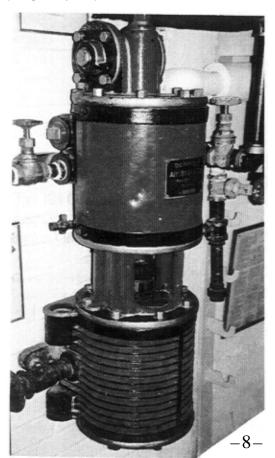
Engine #15 Locomotive Air Compressor
