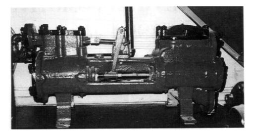
Engine #25 Duplex Cylinder Feedwater Pump
