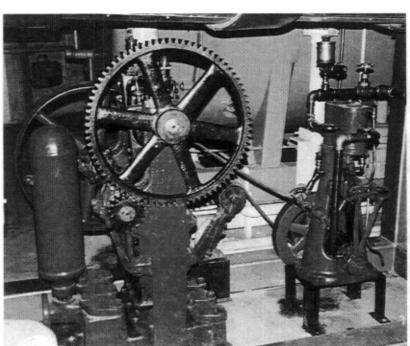
Vertical single-cylinder bottle-frame steam launch engine of 1890s vintage, fitted with Stephenson reverse gear. Engine has cylinder dimensions of 2 1/2" X 3" and is belted to a triplex elevator pump that was manufactured by the Gould Pump Company. Cylinder dimensions of 4" x 6".
