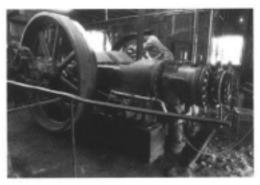
Bessemer engine drives the line shaft through a clutch on the right with the clutch handle shown in the foreground. *Courtesy Doug Box, Doug Box Photography*
