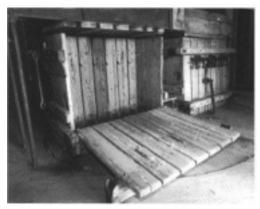
Double box bale press allowed cotton to fill the box on the right while pressing and unloading a bale of cotton from the other box.
