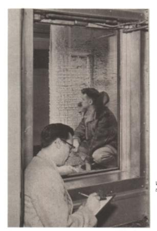
Wing in IRT test section before ice has been shed from a pneumatic boot deicer.
