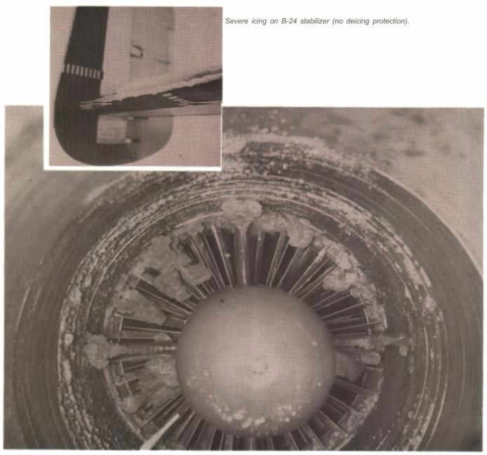
Ice on inlet guide vanes of an early jet engine (no deicing protection)
