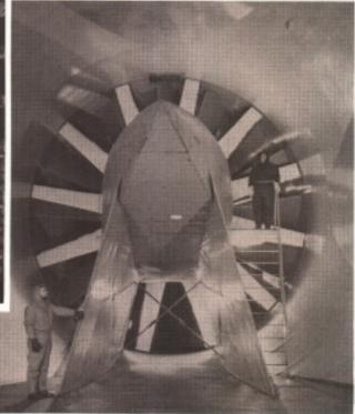
4100-Horsepower drive fan (24-ft diameter) for IRT (looking upwind).
