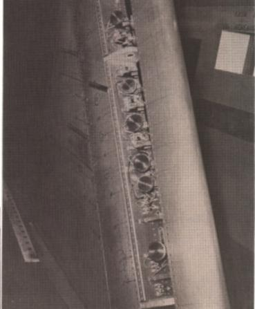
Unique icing problems associated with the helicopter are resulting in many IRT tests by government and industry. The test of the rotor section shown here was to evaluate proposed electrothermal deicing designs.
