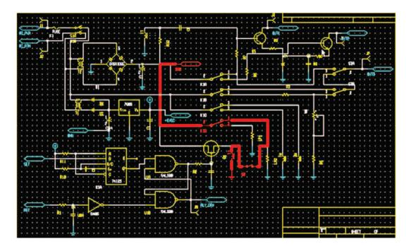
Circuit design with red path indicating a step in the sneak circuit analysis process.
