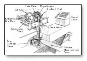
The electrical motors, used to drive the hoist, are designed to operate, up to a maximum required capacity, at a continuous fixed rate of speed regardless of load variations imposed by the distribution of the weight of the vessel. All of the motors are controlled from one central point. In the event of malfunction of any one motor, the entire system is automatically stopped.
