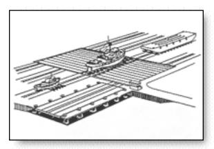
A transfer system can be added to a basic SYNCROLIFT® shiplift by providing railroad or crane-type rails on the platform and on the adjacent land area. The rails are arranged so that a transfer cradle, with a ship on it, can be rolled to the land area when the platform is at the yard elevation. The on-shore transfer system can be designed to permit movement in both directions.
