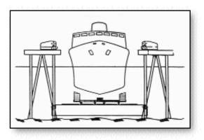
The platform, which supports the vessel during the lifting operation, is raised and lowered by electrically controlled hoists and wire rope cables. The hoists are supported by fixed structures consisting mostly of standard marine piling.
