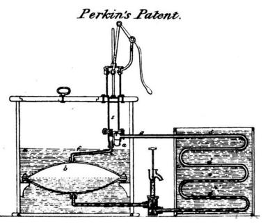
Right: Drawing from Jacob Perkin's patent entitled, "Apparatus and means for producing ice, and in cooling liquids."
