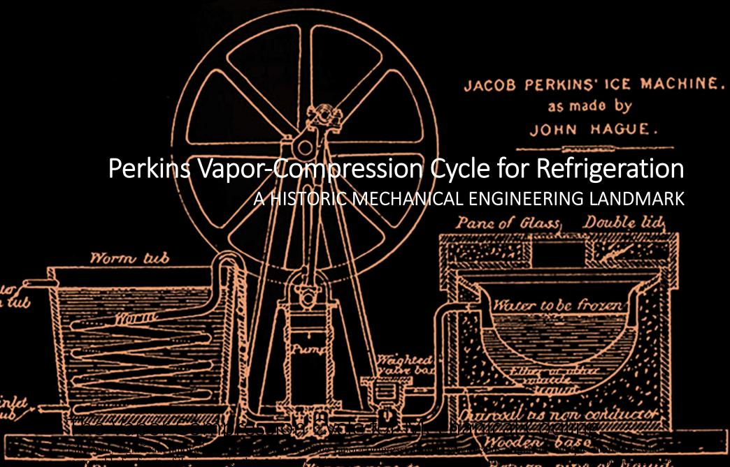
Pipe in continuation of bottom of worm leading to weighted valve box Yapour pipe to suction valve of pump Return pipe of liquid from upper part of weighted valve box
